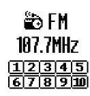
FOR The AUTOMATIC TUNING. PRESS AND HOLD FORWARD OR REWIND BUTTON FOR 2SECONDS. THE TUNNER AUTOMATICALLY SCAN AND STOP ON THE NEXT STATION WITH A STRONG SIGNAL. IN AREA WITH WEAK RECEPTION, PRESS THE FAST FORWARD OR REWIND BUTTON TO FIND A CLEAR STATION.
